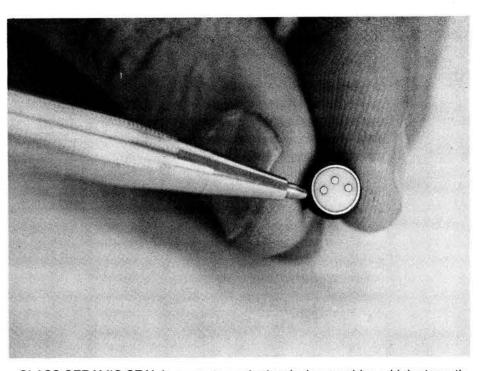
GLASS CERAMIC SEAL in a weapon actuator device provides a high strength bond to the Inconel shell of the actuator and to the electrical pin feedthroughs. The glass ceramic matches the coefficient of thermal expansion of the other materials. The actuators have survived explosive testing to 150,000 psi.
